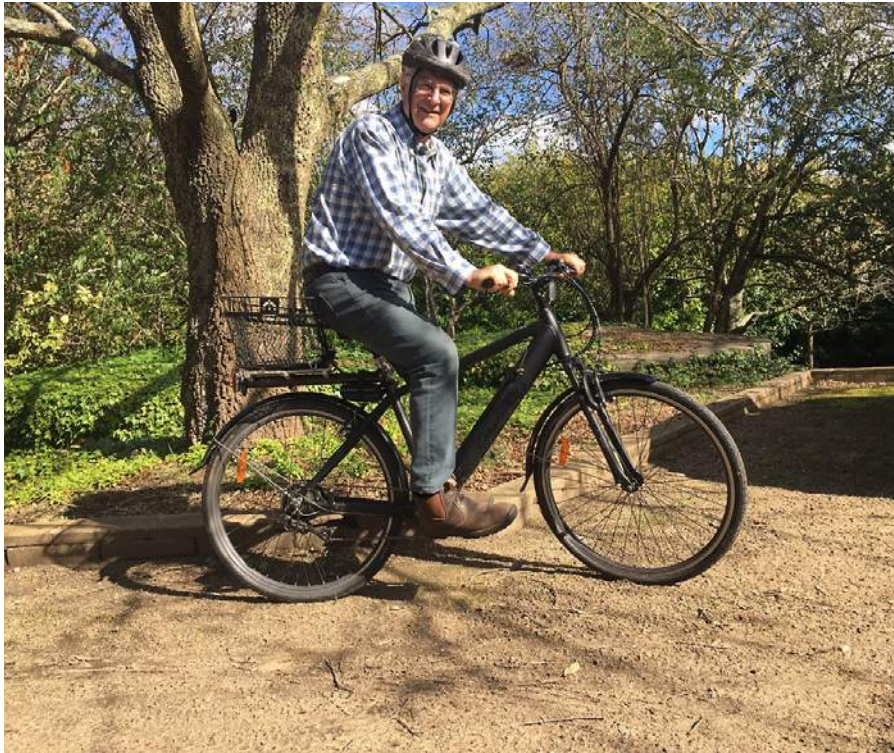
The reporter with the cheapest of them all – a supermarket ebike for $1000 with 28" wheels, 250w rear-hub motor and 7.5Ah, 270Wh battery. It works well until hills become steep. Then it's either pedal harder – or walk and push it uphill!
